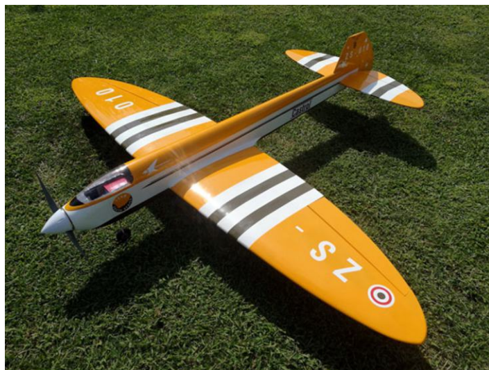
Iconic Novi Arrow III, designed and flown by John Brink. Elliptical planform is most effective, and long fuselage ensured great longitudinal stability.
